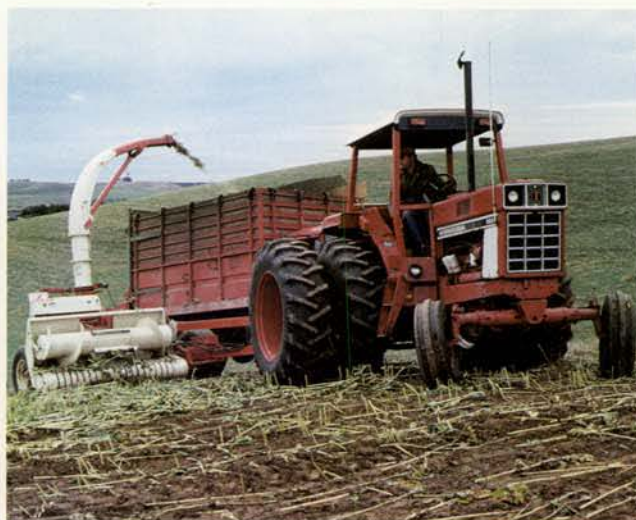
Fig. 2. Row spacing should match harvest equipment to prevent separate cutting and harvest operations as shown here.
