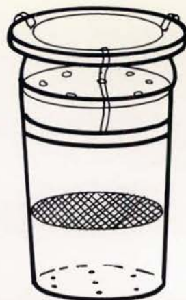
Fig. 8. Release cage for containing knapweed seed heads and associated seed during bioagent release.
