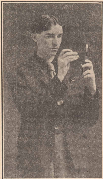
FIGURE 4.—Shows method of holding bottle and dividers while reading the test.
