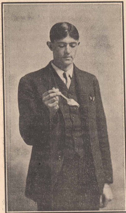
FIGURE 3.—Milk bottle is shaken in order to mix acid and Milk. Care should be taken to point bottle away from face.
