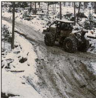
Compact skid trail snow before skidding logs. This avoids damage to soils that are still wet or not completely frozen.
