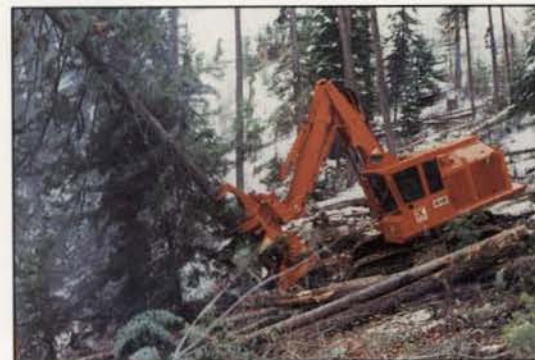
Below: Feller-bunchers are mechanical harvesters that move through the forest and harvest trees and pile them in bunches. They can reach into sensitive areas and thin individual trees without damaging remaining trees, water, soils, or wildlife habitat.
