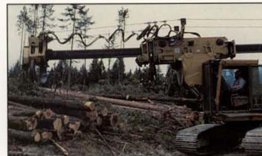
Above Slide-boom delimiters begin the manufacturing process right in the forest. They quickly snip off the branches and cut the stem into exact lengths.
