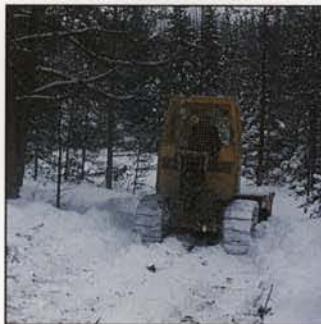
Compact skid trail snow before skidding logs. This avoids damage to soils that are still wet or not completely frozen.
