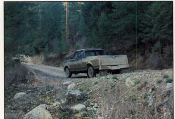
Gradients steeper than 8 percent give collected waters too much momentum and the ability to carry excessive sediment and debris for great distances.
