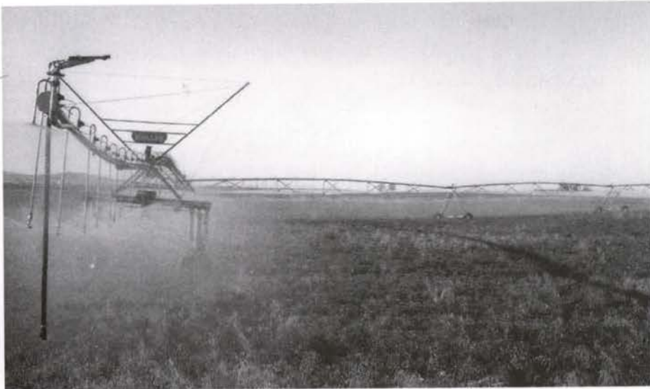
Center pivot with corner system.
