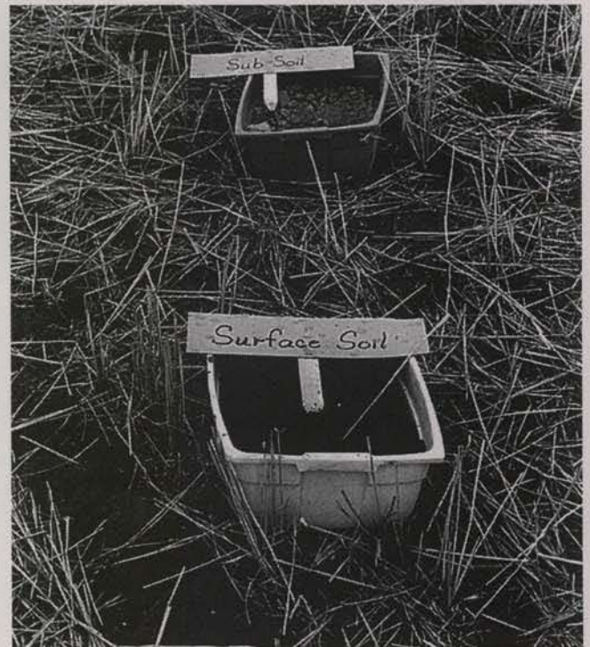
Fig. 4. Some type of container, such as a plastic pan, will be used at each site to hold samples of surface soil and subsoil material. This ensures that all participants will be considering the same horizon of the exposed soil profile.
