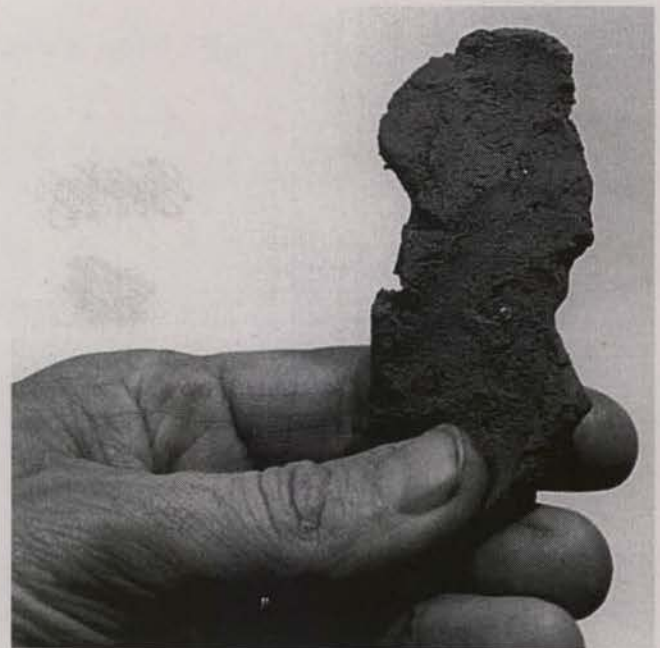
Fig. 11. A silty clay textured soil, with 2 percent sand, 54 percent silt, and 44 percent clay, can be squeezed up and between thumb and fingers to form a ribbon 2 to 3 inches long before it breaks.
