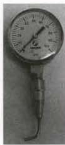
Figure 4. Pitot tube attached to pressure gage that is used to measure operating pressure of a sprinkler nozzle.
