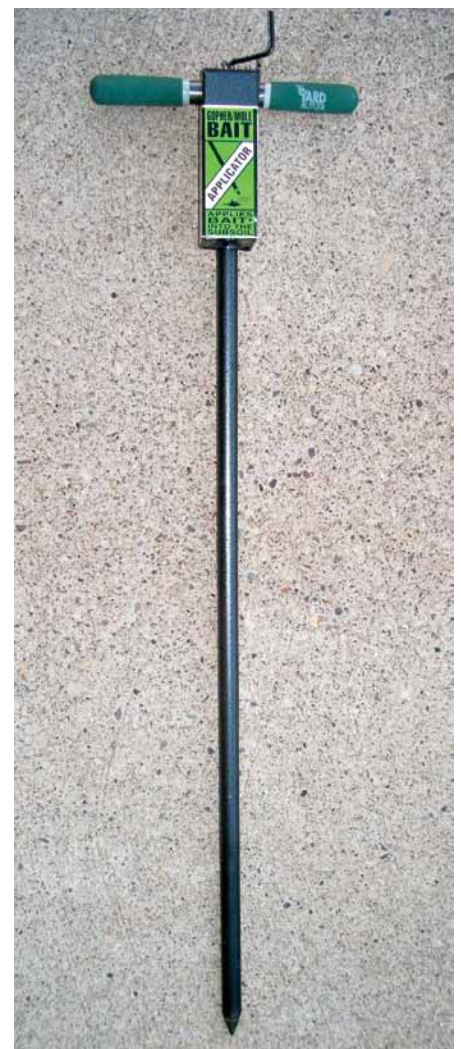
Figure 20. Hand-held gopher baiting apparatus. Photo by Danielle Gunn.
