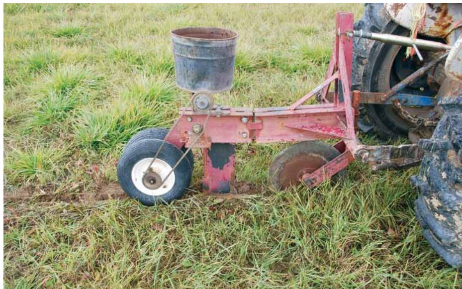
Figure 22. Burrow builder applicator. Photo by Glenn Shewmaker.
