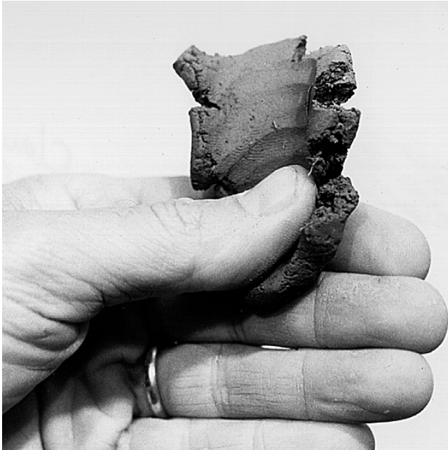
Fig. 10. A silty clay loam textured soil, with 3 percent sand, 68 percent silt, and 29 percent clay, forms a smooth ribbon about an inch in length before it breaks off.
