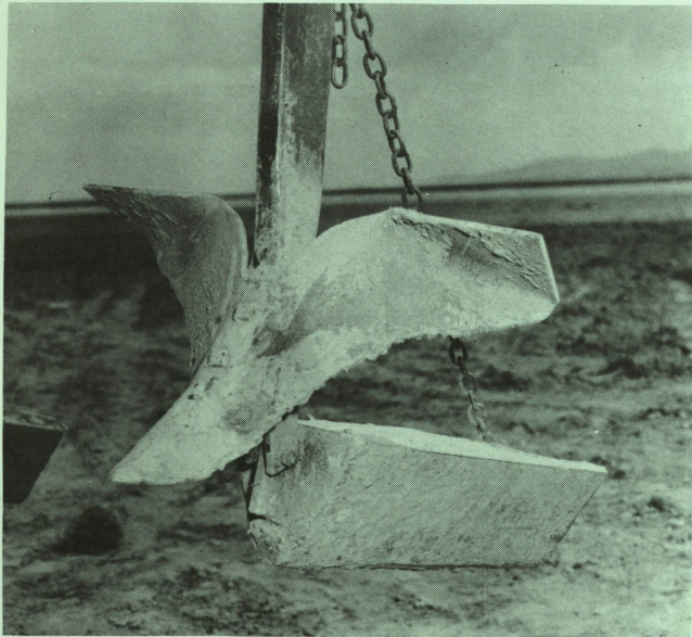
Figure 4. Furrow slickers smooth up the bottom and sides of the furrow decreasing the water intake rate. This moves water across the field faster, allows longer runs, gives more even distribution.
