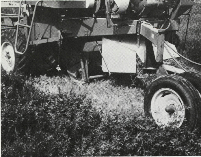
Figure 1. Experimental machine illustrating the position of the spray nozzle.
