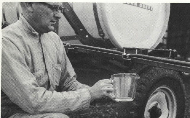
Figure 1. Measuring the flow from an individual nozzle.
