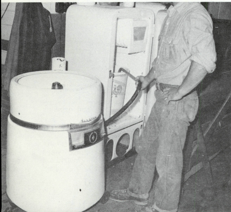
Figure 3. Conventional type washing machine used to mix warm water with milk replacer powder. Machine pump and hose transfers mixed milk to refrigerator storage container for cooling.
