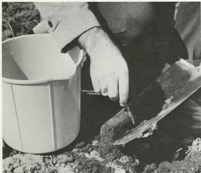
3. Taking a sub-sample with a shovel. Cut 1/2 x 1/2 inch core out of soil slice.
