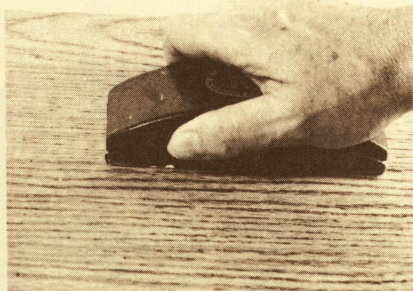
Sand the wood surface with the grain of the wood.
