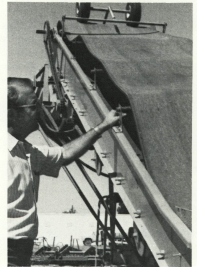
Fig. 8. Anti-roll belt on side elevator (right) permits removal of flights, prevents rollback and helps remove dirt.
