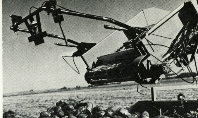
Fig. 10. Sensor used in the automatic boom height control.
