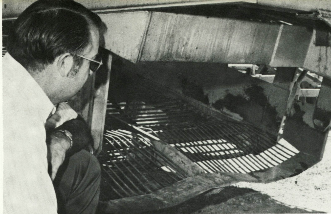
Fig. 2. The vibrating blade (above) oscillates about a rubber bushing in the center.
