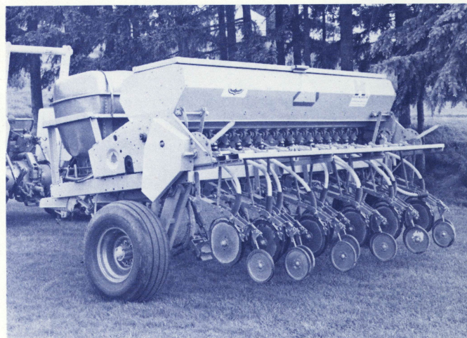
Fig. 1. The 1977 prototype Chisel-Planter from the rear showing the grain box, double disk openers and press wheels.
