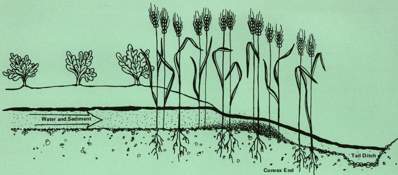
Fig. 3. A filter strip works on the principle that the less energy a stream of water has, the less sediment it can carry. When runoff water carrying sediment enters the filter strip, the stream slows down and spreads out. Extra sediment that can no longer be carried settles out while water continues on through to the tailditch.
