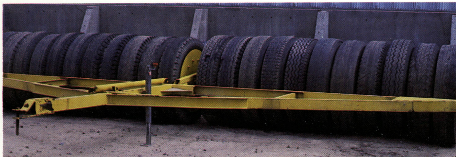
Fig. 4. Homemade vine roller for 6 rows wide.
