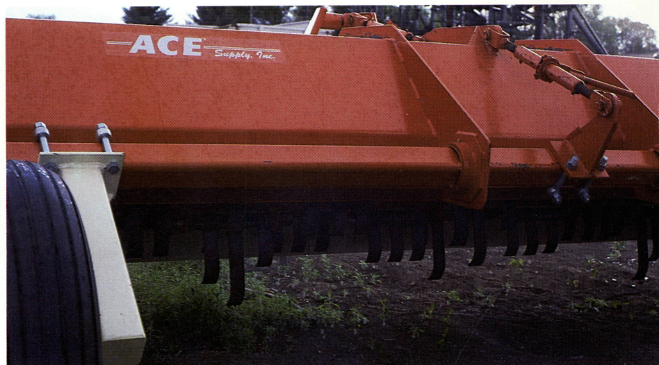
Fig. 3. Potato vine flailer with contoured metal flails.
