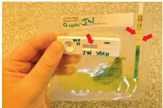
Figure 1. Two types of test kits (one well and one strip) used for diagnosing PVY and PVY N . Note the quarter-sized sample of macerated foliage in the pouch with buffer. The test strip shows a positive (control line at top and test line at bottom) result for PVY. The well-style kit (white plastic tray) indicates a negative test (control line but no test line) for PVY N . Laboratory results verified the sample to be PVY N:0 .
