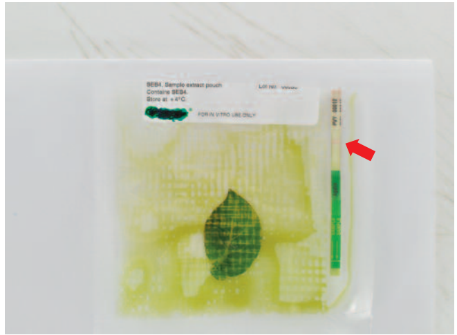
Step 4. Place the strip into the pouch sample-end first. Submerge no more than \frac{1}{4} inch of the strip in the extract. Wait up to 30 minutes for test results. One red line (as above) indicates the test worked but results are negative. Two red lines indicate a positive result. No line indicates a faulty test.
