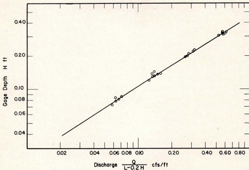
Figure 7.—Gage depth-discharge relationship for flow over a contracted weir.
