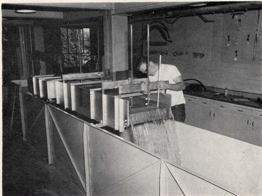
Figure 2.—Gage reading being taken on suppressed weir.
