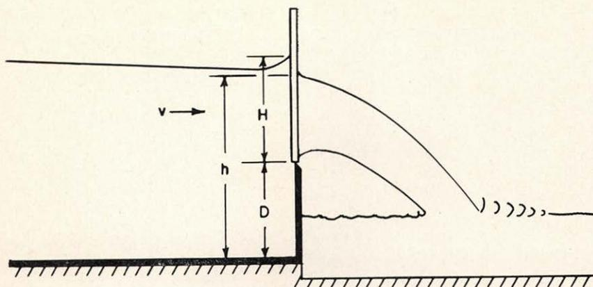
Figure 1.—Gravity flow over a sharp crested weir with a gage held on the crest.
