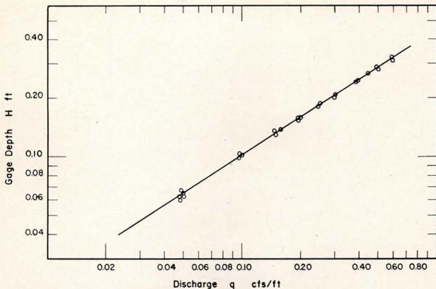
Figure 6.—Gage depth-discharge relationship for flow over a suppressed weir.
