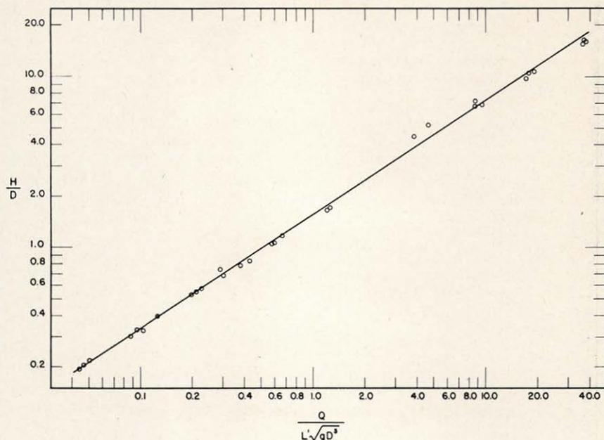
Figure 5.—Relationship of dimensionless grouping of variables for contracted weir flow.
