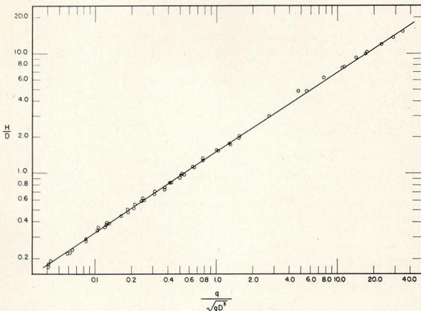
Figure 4.—Relationship of dimensionless grouping of variables for suppressed weir flow.
