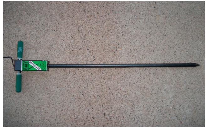
Figure 4. Handheld gopher baiting equipment. Photo by Danielle Gunn
