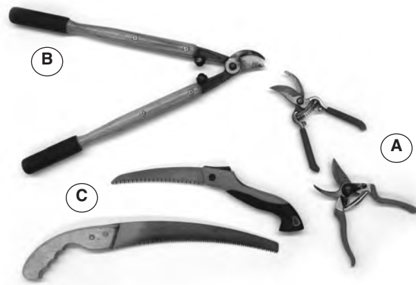
Figure 4. Tools used to prune woody plants include (a) by-pass hand shears, (b) by-pass loppers, and (c) hand saws. Photo by Robert Tripepi.
