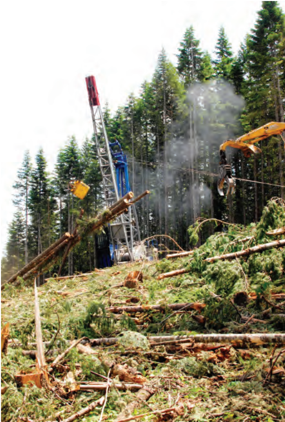
Feller-bunchers fell, limb, and cut logs to length at the harvest location.
