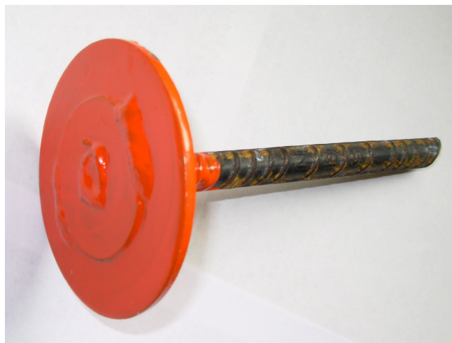
Figure 2. Example of a welded stake. Discs on top are metal washers and are welded to a piece of rebar cut at an angle. Discs were painted with orange implement paint, which doesn't degrade as quickly as other types of paints.
