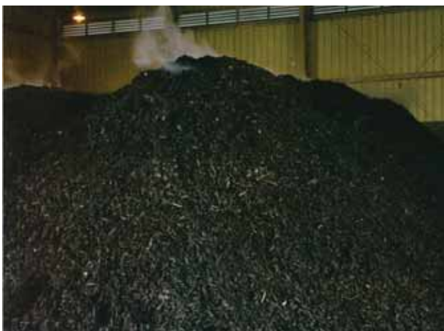
Figure 5a. Municipal composter involves composting in an aerated 3-sided and roofed structure leaving the front wall open for delivery and pick-up of compost.
