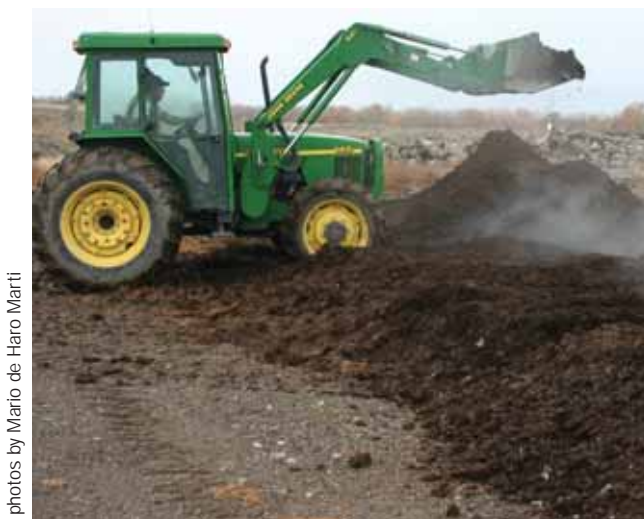
Figure 1. Mechanically turning compost with tractor—the turned-pile method of composting—works well for farmers who can use tractors to turn a pile, adding porosity lost during settling.
