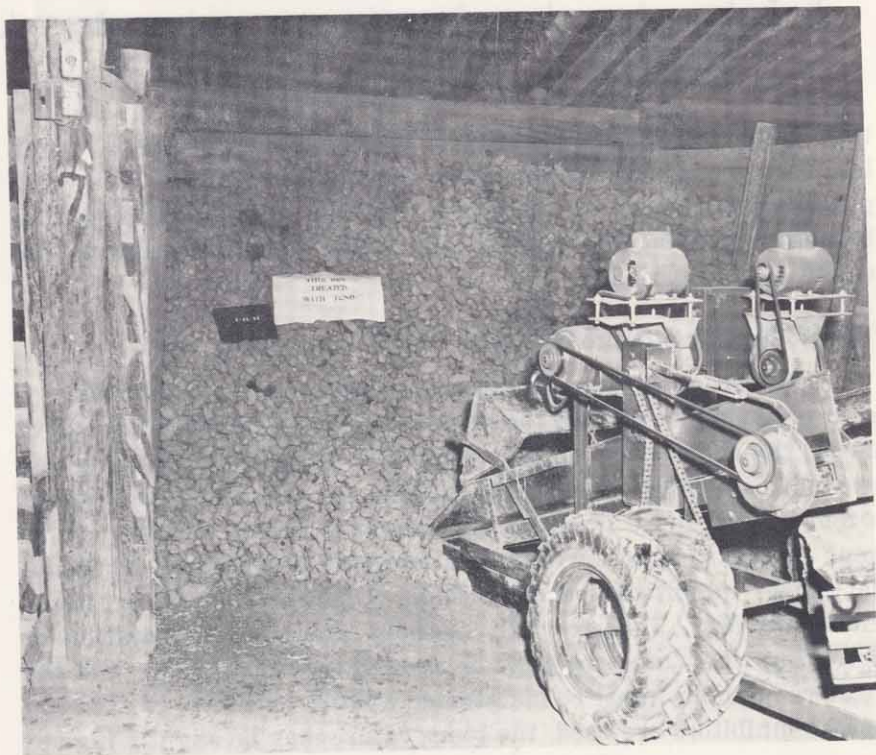
Figure 11. The mechanical scoop conveys the bulk potatoes from the storage cellar to a bulk truck.
