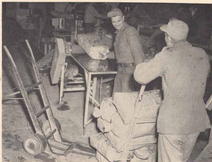
Figure 15.—Loading a hand truck with the aid of a power conveyor and loading table. This system eliminates the lifting of each sack from floor level. It also assembles sacks at a central loading point.
