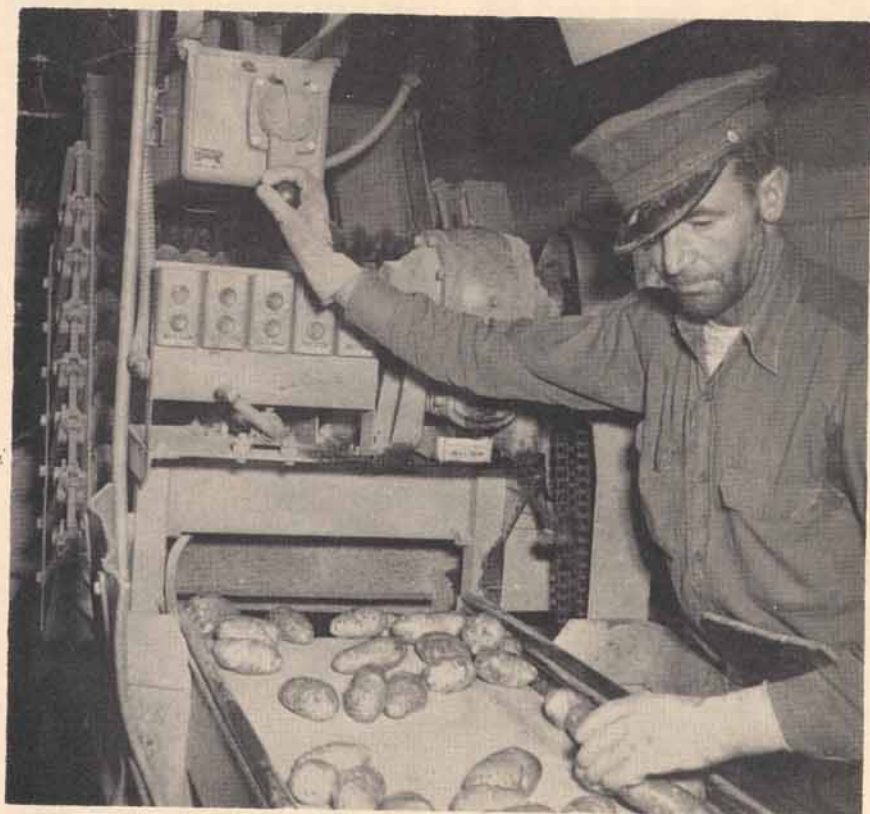
Figure 9.—A remote control unit for regulating potato flow to the packing line. Such a convenient location allows the head grader to adjust potato flow with changes in potato quality. Stop-start switches for all drive motors in the packing line are within easy reach of the head grader.
