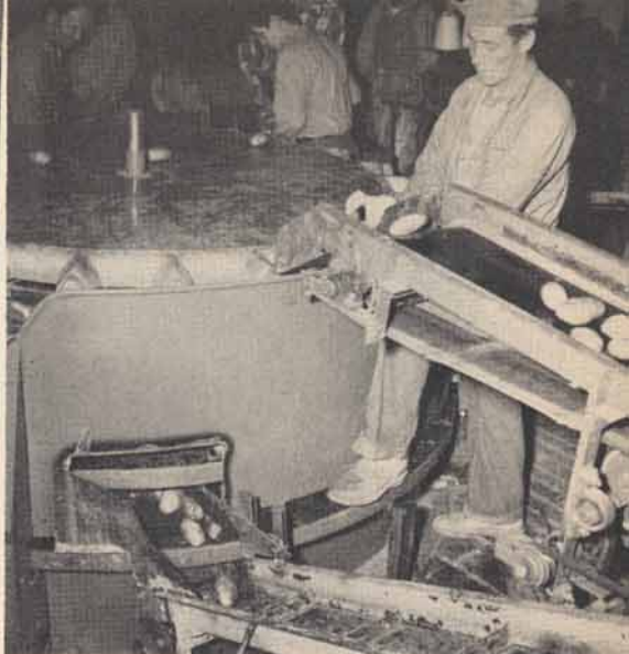
Figure 14.—A bagging wheel designed and built in an Idaho plant. This bagger features a conveyor to return over-flow potatoes to supply conveyor for re-feeding. The wheel is rotated by the feet. This frees both hands to adjust the bag fill-level.
