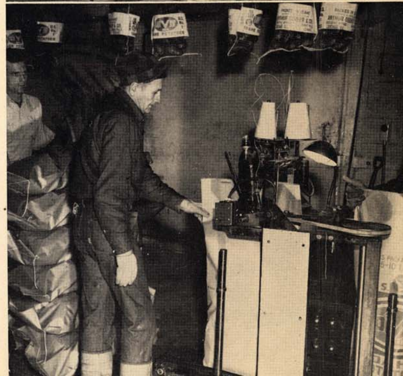
Figure 11—Mesh sacks dropping to baling crew from monorail hooks. Little automatic devices such as this save much hand labor.
