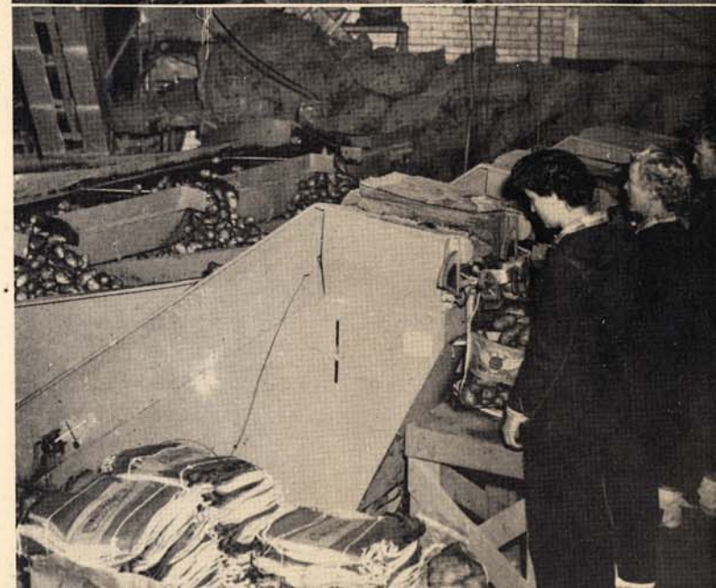
Figure 6—(Lower) Automatic tub machines in operation. Each tub holds a small reservoir of potatoes for the two sack fillers. This was found to be a low cost method of filling sacks.
