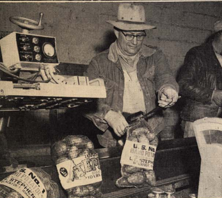
Figure 7—Automatic stapling operation on a monorail. This is a fast, low-cost method of closing mesh sacks.
