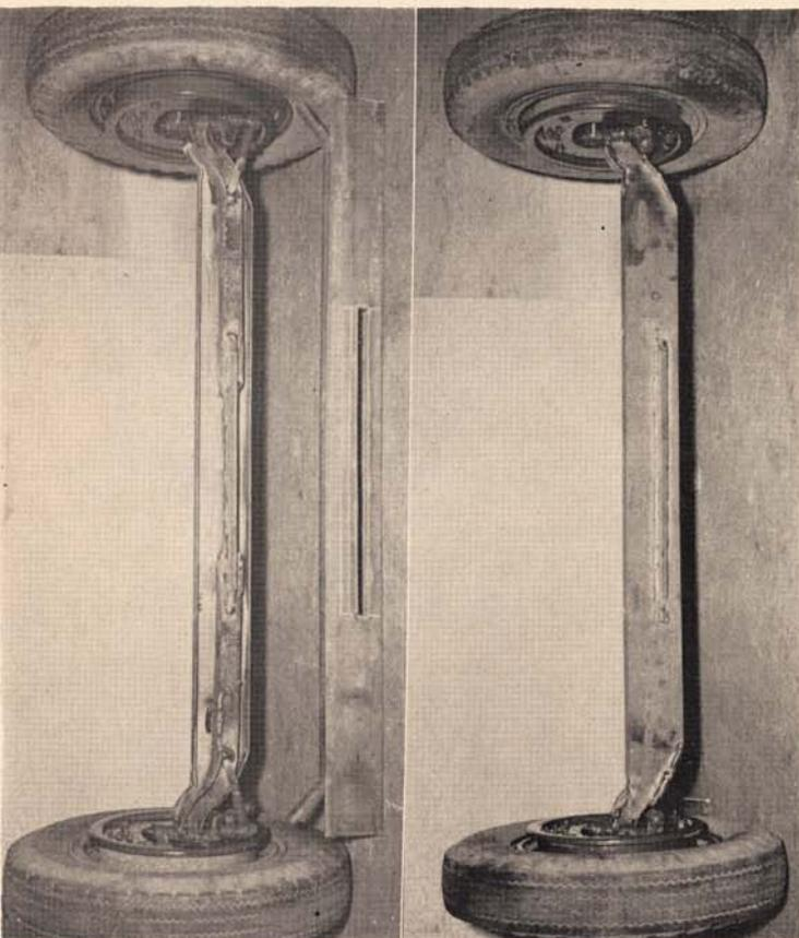
Figure 4.—A second-hand truck front axle was altered to serve as the rear axle for the implement carrier. The upper picture shows how the axle was cut, spaced with bar steel, and then reinforced with 6-inch channel iron. Note how the tie rods to the steering arm were welded to the axle. The bottom picture shows the completed axle. Care should be used to maintain a slight toe-in and the original camber of the wheels.
