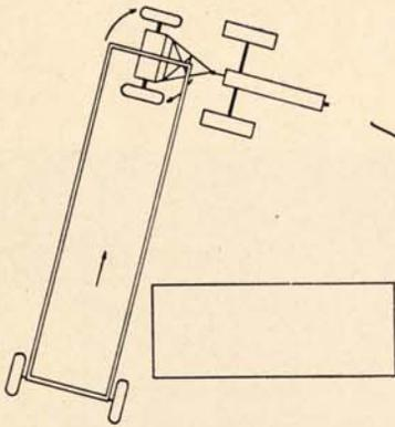
Figure 1.—A sharp turn as shown is required to position the implement carrier over a load. The turn is made when the rear wheel nearest the load is in position.
