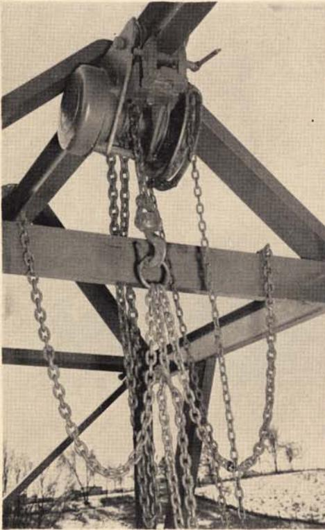
Figure 2.—Geared chain hoists on trolleys are used to lift the load. Three chains attached to a ring are looped over the hoist hook to lift the load.
