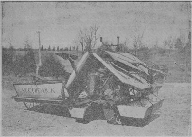
FIG. 1—A grain binder equipped with pans and with extension to the rear elevator plate and binder deck. This arrangement saves the clover seed that shatters in cutting and binding. (Courtesy United States Department of Agriculture.)
