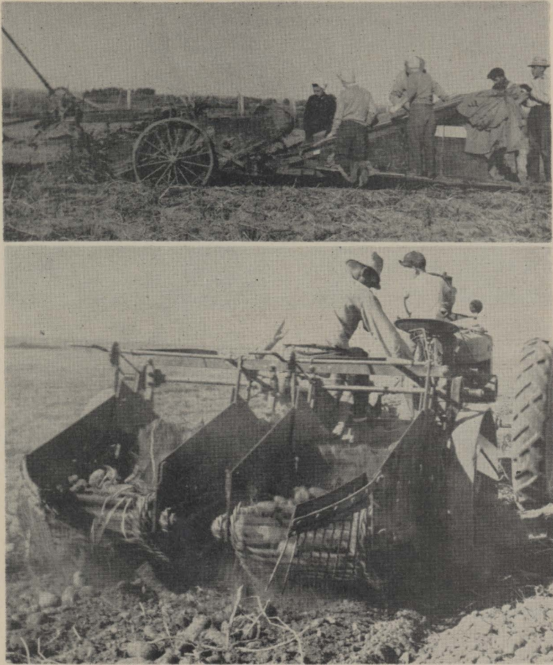
Figure 2. (A) trailer-type digger-picker, (B) two-chain level-bed digger.
