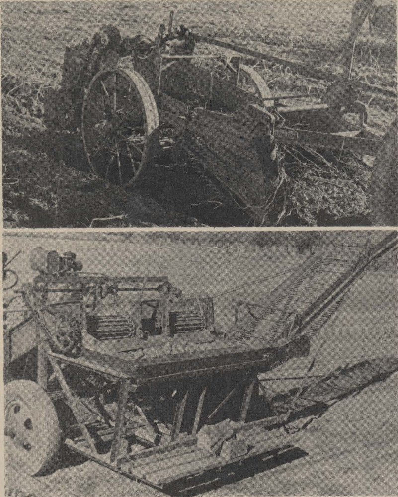
Figure 7. Additional types of mechanical harvesters used in 1949, (A) single-chain level-bed digger, (B) rubber-roller bulker-combine.
