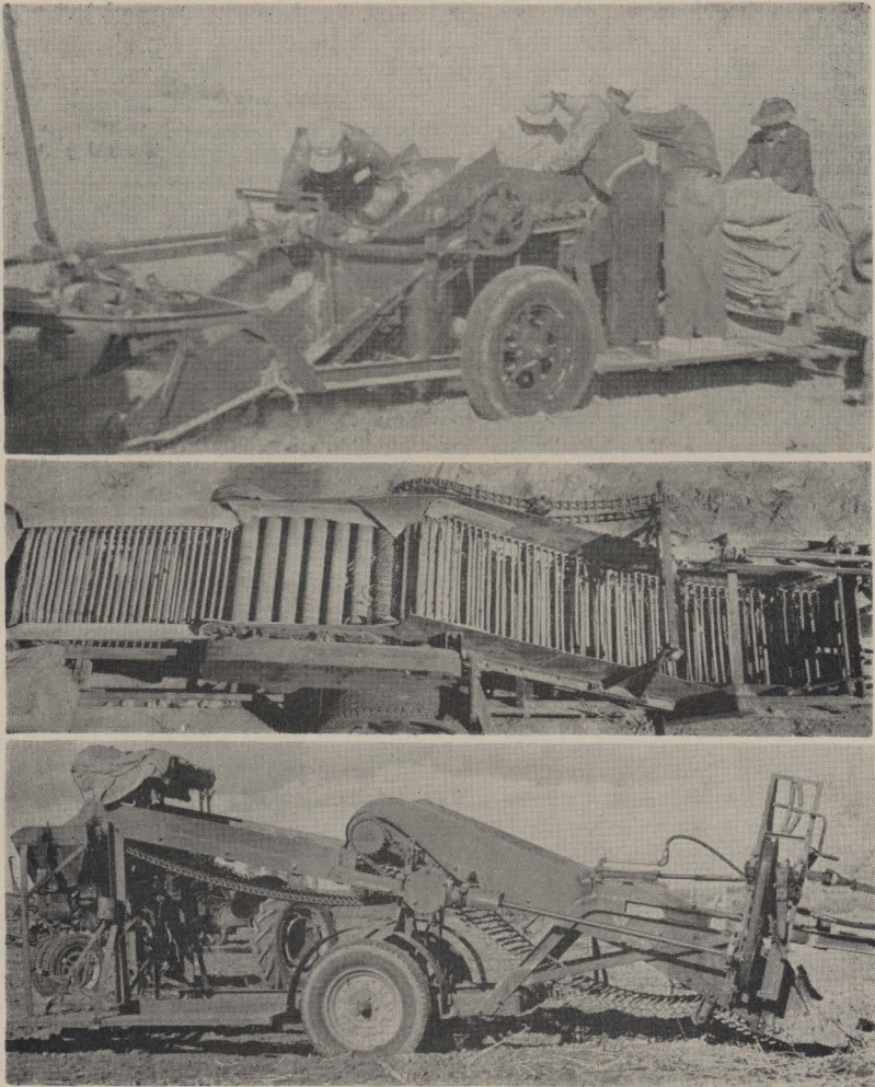
Figure 6. Two types of harvesting machines used in 1948 that were not used in 1947, (A) side view of rubber-roller digger-picker, (B) top view of rubber-roller digger-picker, (C) non-rubberized digger-picker.
