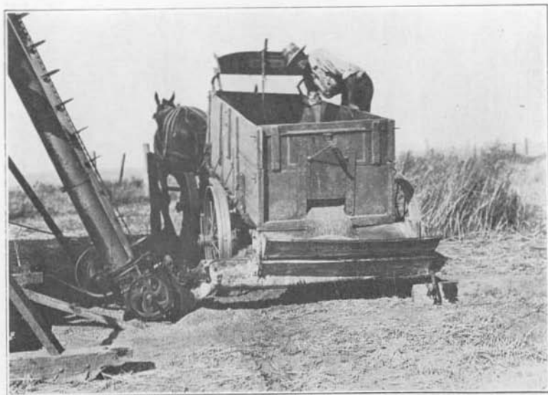
Portable type elevator, employing endless chain and drag links, operated by a three horsepower gasoline engine. Note end delivery into movable elevator hopper, also power lift for gravity dump.
