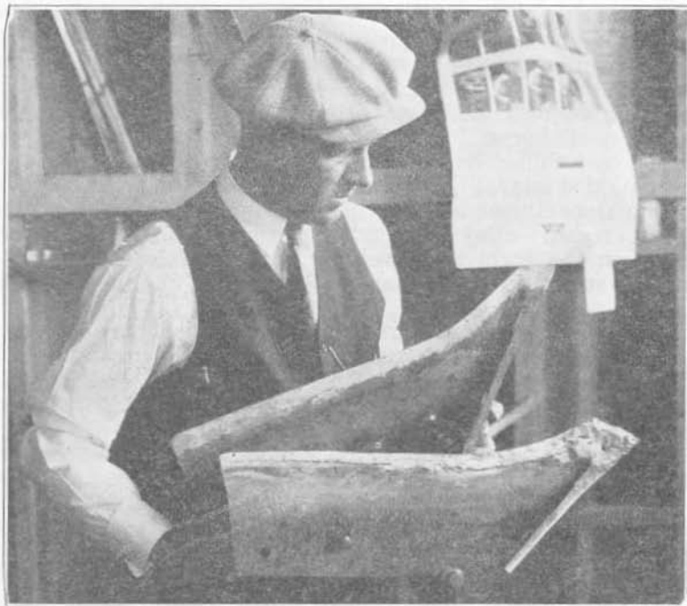
Plowshare prepared for alloy treatment and treated plowshare in special vise.
