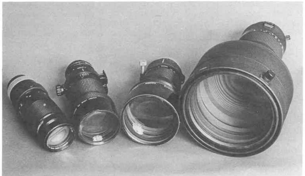
All the lenses are 300mm (6 power) lenses. From left to right: f5.6 ($200) f4.0 ($350-400) f2.8 ($1,000-1,500) f2.0 ($4,000)—this one weighs about 12 pounds.
