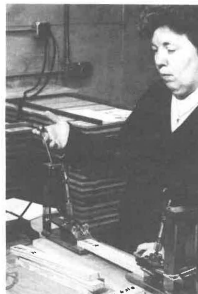
Evaluation of strength properties of fire-retardant-treated material after exposure to elevated temperatures.
