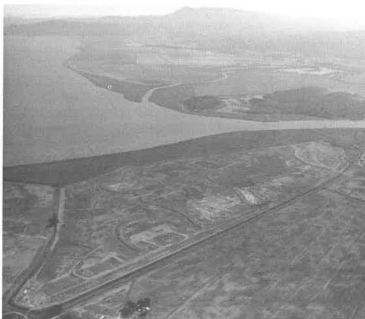
Marsh restoration site with new levees and channels, before the addition of dredged materials. A natural marsh extends between the bay shore and the site at the mouth of the Petaluma River. To the right is Highway 37 and Port Sonoma-Marin.
