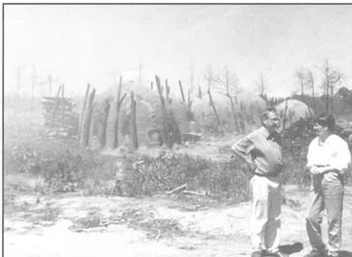
With a forest plantation owner in Minas Gerais, Brazil. Pinus caribaea is harvested for sawlogs and charcoal. Charcoal ovens are in the background surrounded by bolts. The clay ovens are loaded to the top with wood, ignited and allowed to burn slowly. The charcoal is then hauled to nearby steel mills.
